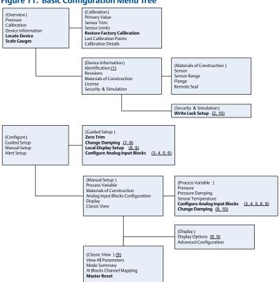
Figure 11. Basic Configuration Menu Tree
